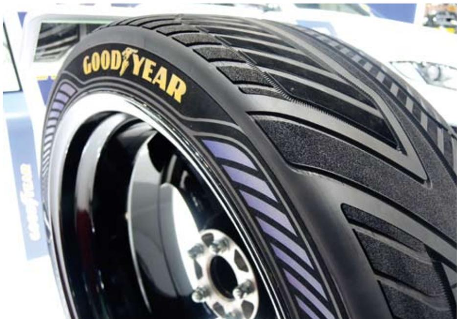
The concept tyre IntelliGrip is supposed to equip early generations of self-driving vehicles with the latest sensor technology in order to support monitoring systems of autonomous vehicles.
