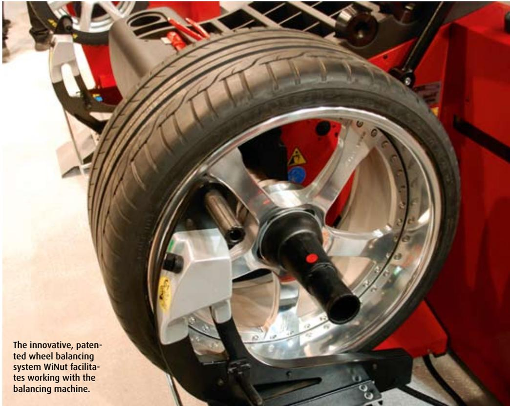
The innovative, patented wheel balancing system WiNut facilitates working with the balancing machine.
