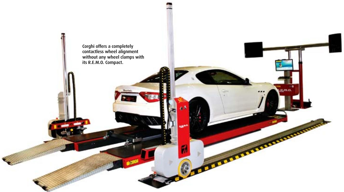
Corghi offers a completely contactless wheel alignment without any wheel clamps with its R.E.M.O. Compact.
