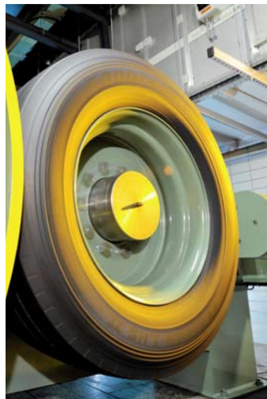
Checking the rolling resistance is already a frequently adapted testing method.
